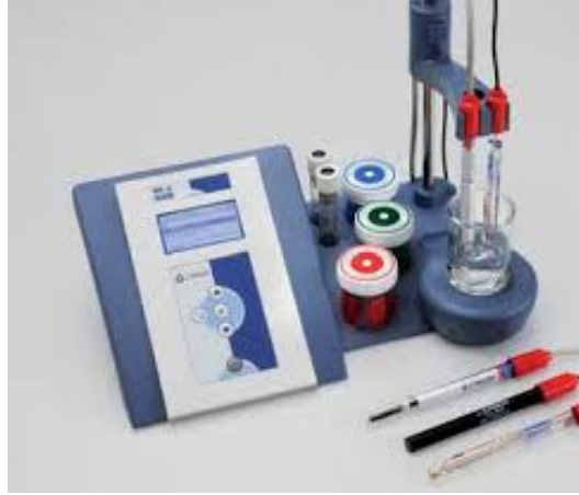
Figure 3.2. Crison GLP 31 device equipped with sodium and chloride ion-selective electrodes.
