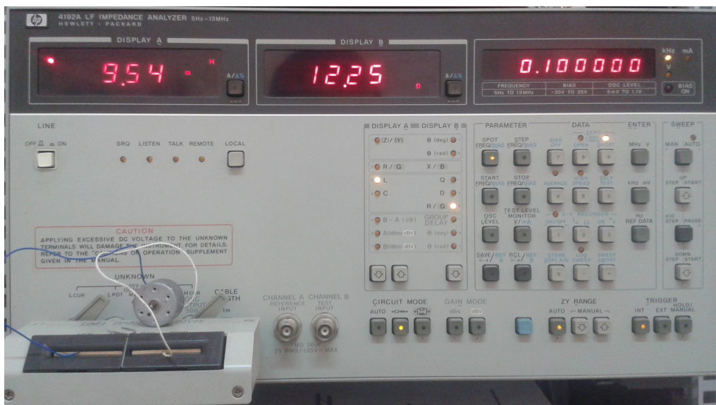
Figure 5.12 – Measuring MDN3BT resistance and inductance
