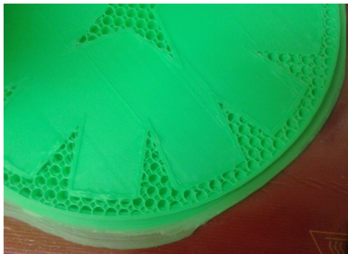
Figure 5.41 – Failed printed part
