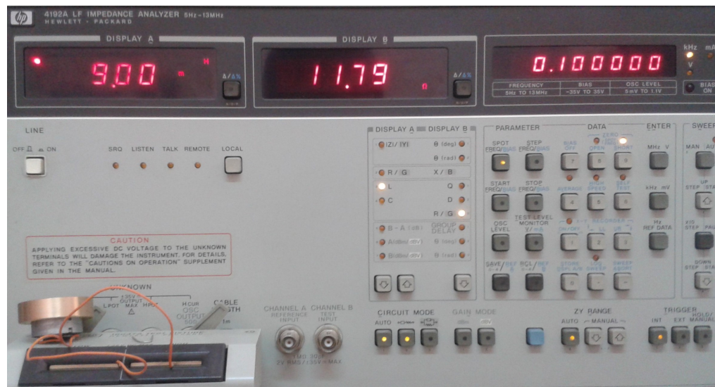
Figure 5.14 – Measuring the motor without name resistance and inductance
