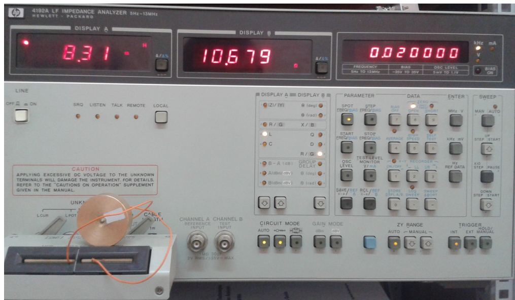
Figure 5.13 – Measuring RF300-CH resistance and inductance
