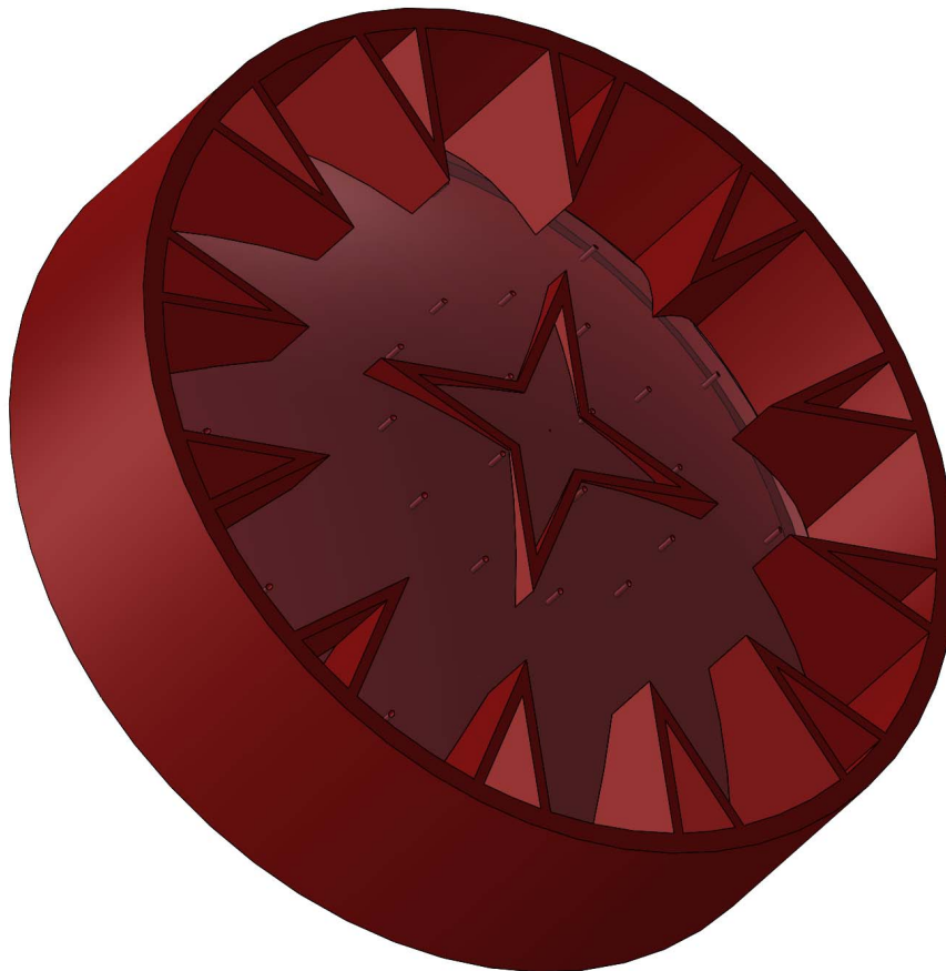
Figure 4.37 – Air-bearing section to show the support triangles
