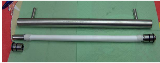
Figure 3-4: Outer and inner tubes constituting the humidifier. The inner one is a high density porous PTFE (polytetrafluoroethylene) tube and the outer tube is made up of stainless steel.
