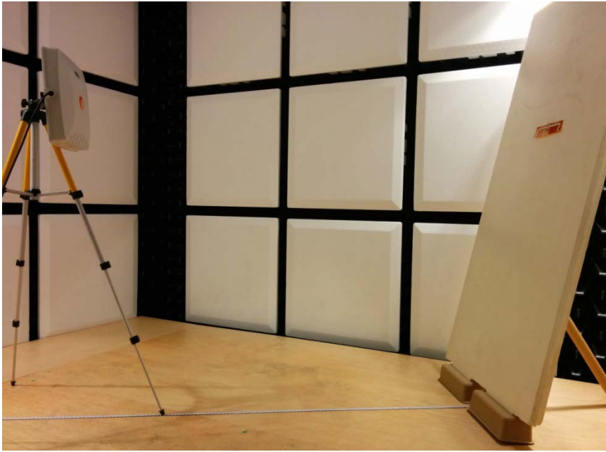
Figure 28. Measurement setup in an anechoic chamber to validate the proposed RFID system. The reader antenna can be seen on the tripod and the smart RFID tag can be observed attached to the foam structure.
