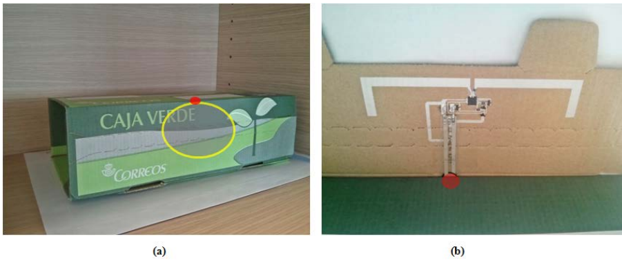
Figure 87. a) Close cardboard with RFID tag; (b) view of the RFID tag before closing the box.
