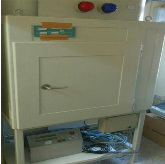
**Figura 12.** Irradiador experimental Yxlon Smart Maxishot 200-E
