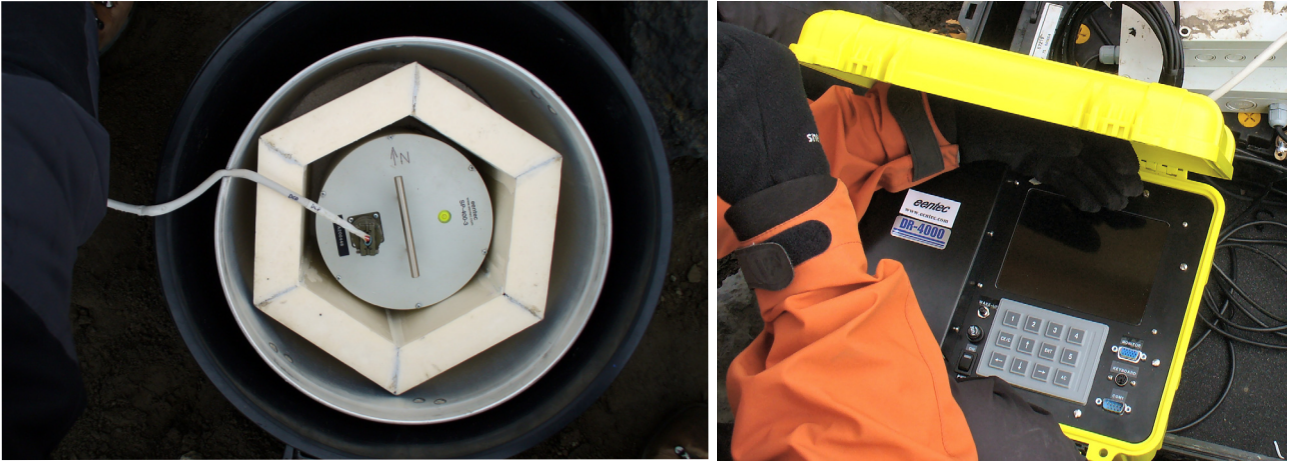
Figure 12. Seismometer (left) and data acquisition system (right) of the permanent station DCP, installed in February 2008 at Deception Island.
