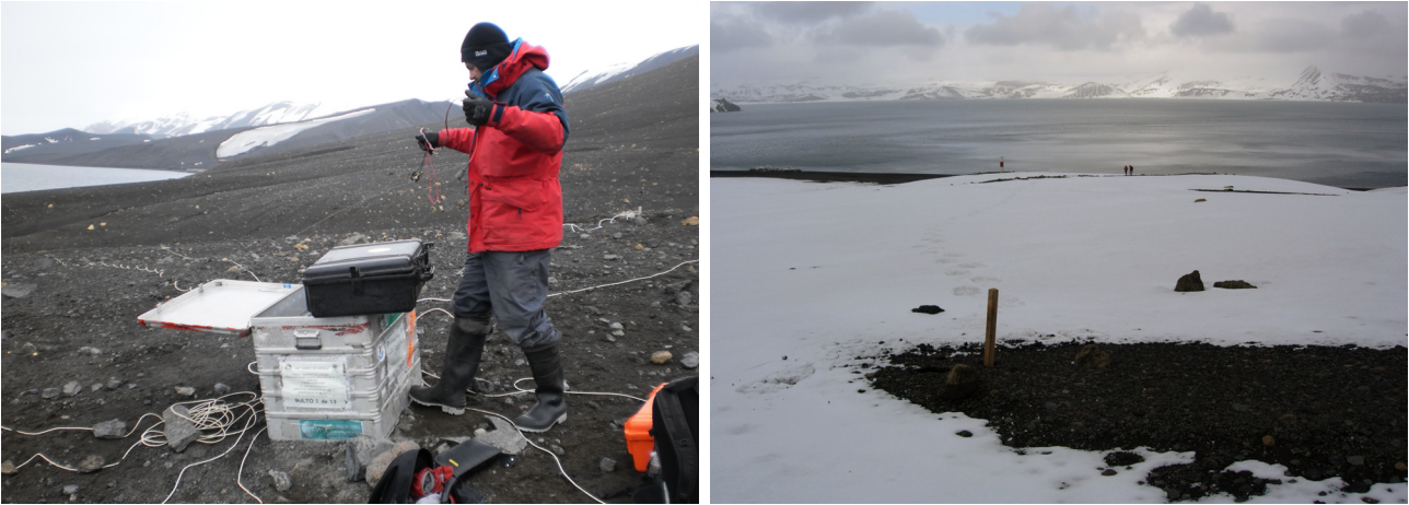
Figure 9. Left: installation of the array data acquisition system in the Fumarole Bay area during the 2010-2011 survey; right: reference stake indicating the position of one of the seismometers of the 12-channel seismic array deployed in the Fumarole Bay during the 2009-2010 survey.
