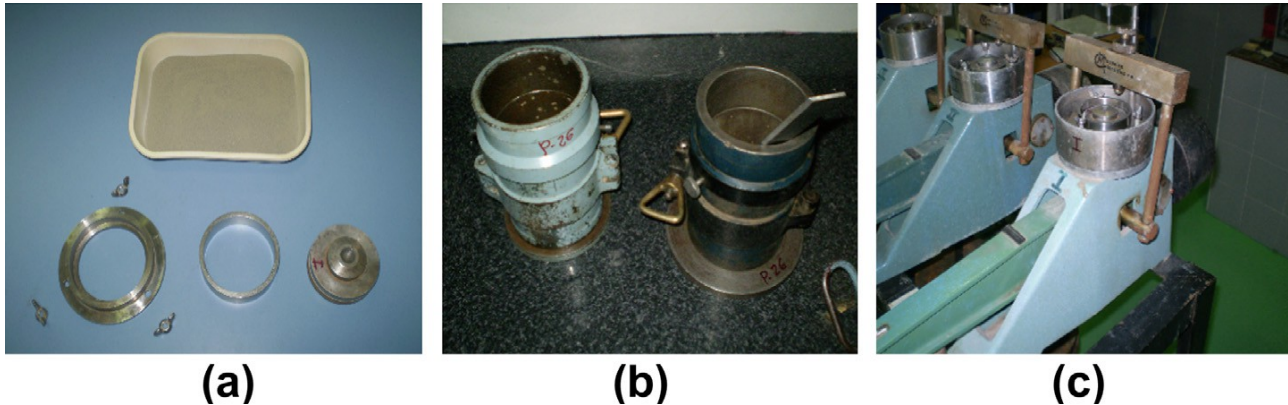
Fig. 6.2. Pictures of lab equipment: (a) preparation of swelling pressure cell; (b) molds for standard Proctor test; (c) oedometers
