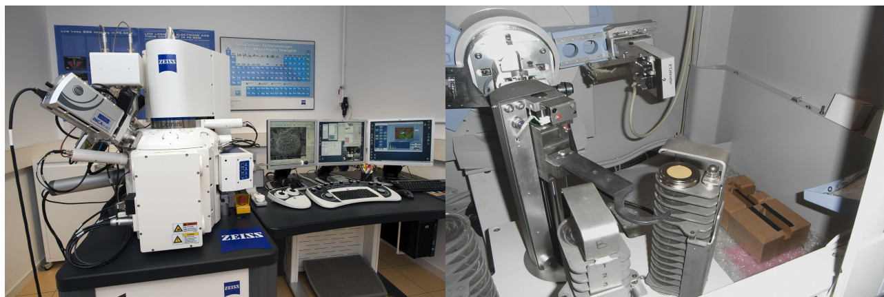
Fig. 7.2. Lab equipment used in this study (University of Granada, Spain): a) Field Emission Scanning Electron Microscopy; b) Phillips X'Pert diffractometer
