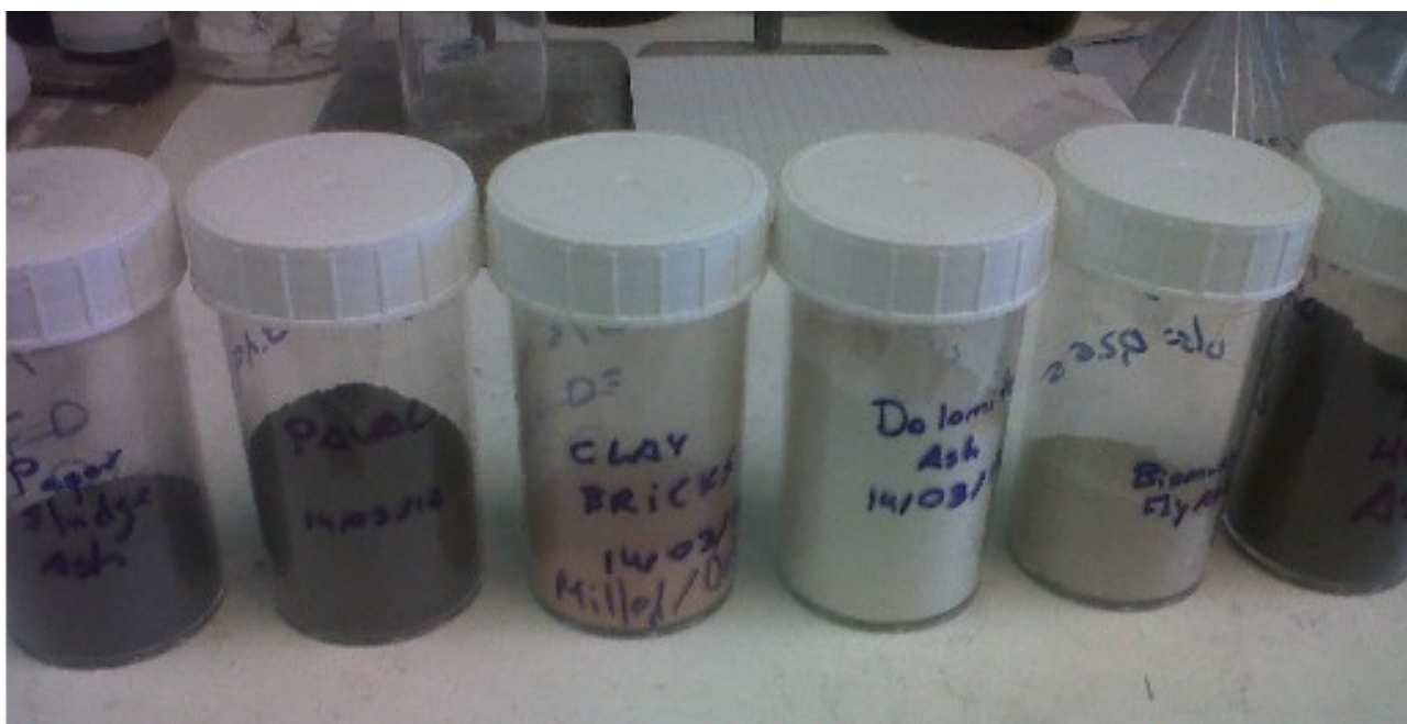
Figure 6.6 Lab picture of the test pozzolans stored in a sealed plastic bottles
