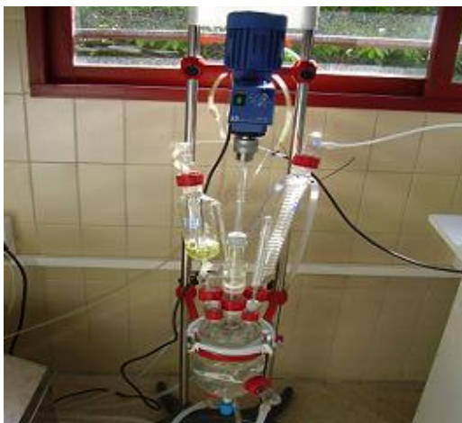
Figure 8. Reactor used for the synthesis of magnetite particles (Laboratory of Department of Applied Physics, University of Granada).
