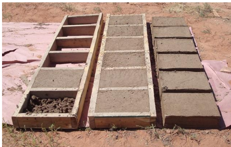
Figure 1-9. Different stages of the manufacturing of adobe bricks ( www.communityrebuilds.wordpress.com ).
