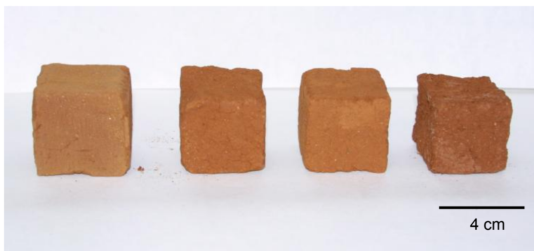
Figure 3-223: Color change of adobe blocks upon alkaline activation (from left to right, untreated, NaOH, KOH and \text{Ca(OH)}_2 ).
