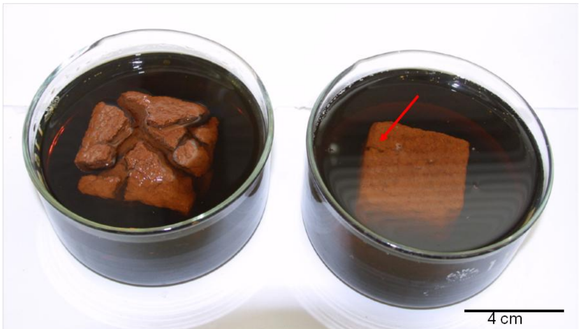
Figure 3-220: Samples treated with NaOH (left) and KOH (right) immersed in water for 48 hours. The formation of fissures led to a complete disintegration of the sample treated with NaOH. The block treated with KOH showed the beginning of crack formation (arrow).
