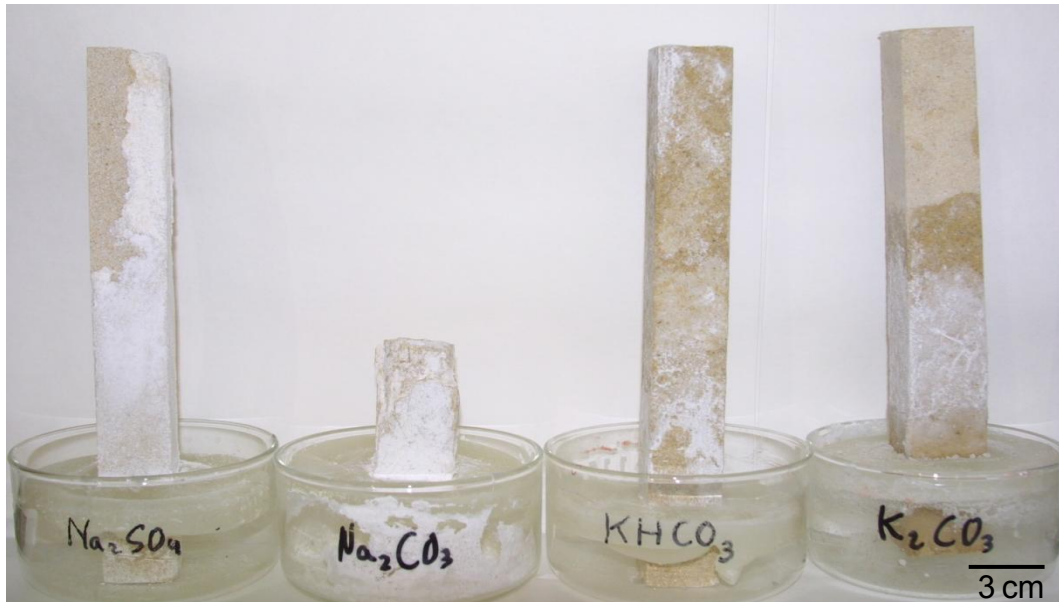
Figure 3-229. Aspect of calcarenite blocks after the removal of efflorescence and loose stone pieces.
