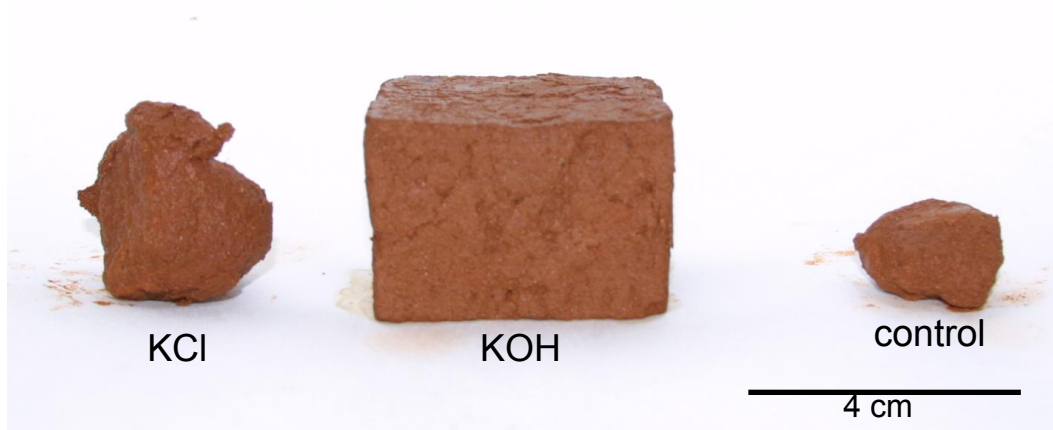
Figure 3-221. Untreated adobe block (control) and blocks treated with 4.65 M KCl (saturated KCl solution at 20 °) and 5 M KOH after immersion in water for 2 hours.
