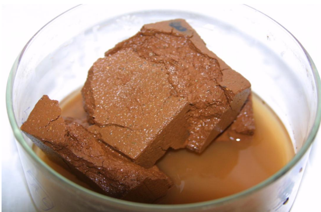
Figure 3-206. Adobe block treated with ethyl silicate and immersed in water for 4 hours (Romero Jimenez 2013).
