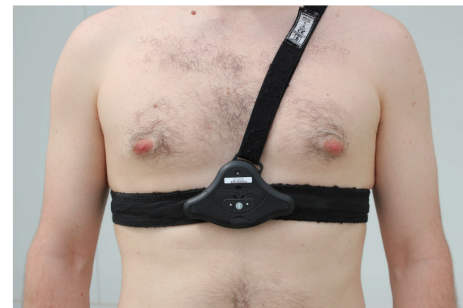
FIGURE 2: Equival LifeMonitor device. It comprises the sensor electronics module (SEM) and the monitoring belt. The SEM contains a battery, electronics, and software, in order to process the measurements from the monitoring belt. The monitoring belt holds the SEM onto the body and contains fabric electrodes, which require contact with the user's skin to measure the body's vital signs.
