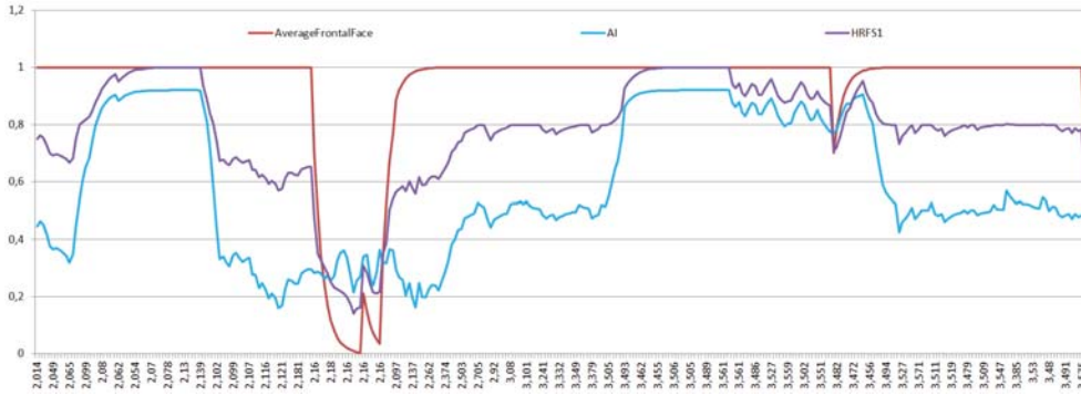
Figure 5.15: Graph showing HRFS1(P) depending on input variables AverageFrontalFace and AI values (Y axis). The X axis represents the distance to the robot (always higher than \beta meters for this case which represents the far situation).
