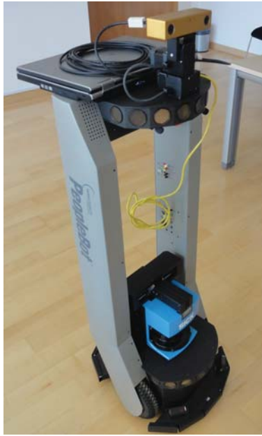
Figure 2.1: Peoplebot robot with a laptop and the Bumblebee stereo camera on the top.
