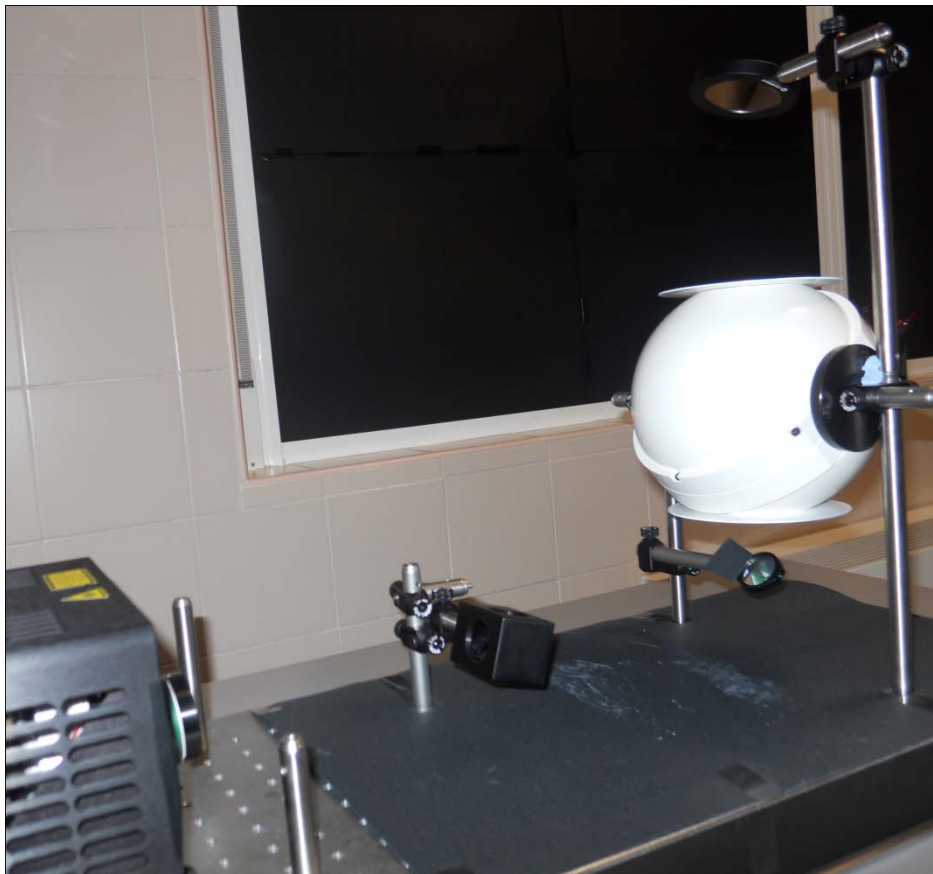
Figure 4.6. Experimental setup used in reflection and transmission measurements on the dental biomaterials. A folding mount allows mirror 1 (bottom left) to be lifted away so that the beam reaches mirror 3 (bottom right) for reflection measurements.
