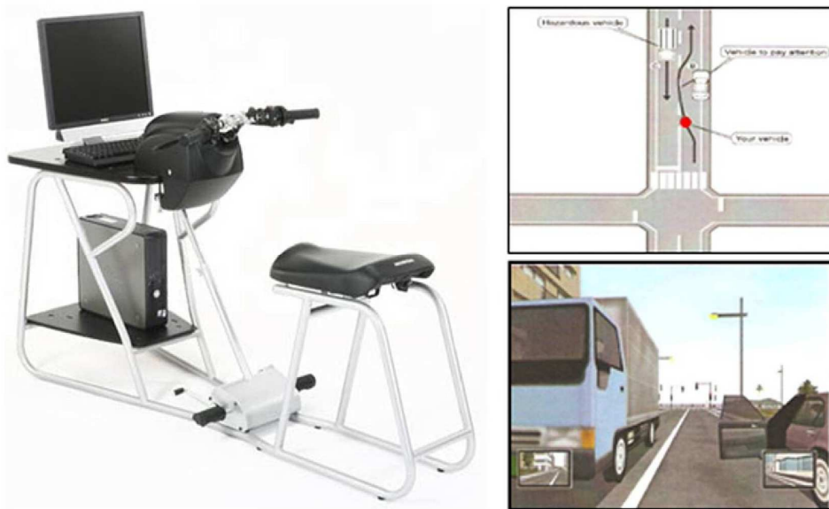
Figure 1. The Honda Riding Trainer (left): this static low-cost simulator is used mainly to improve hazard awareness and perception skills. An example of a hazardous traffic situation presented to the participants (right). Up: schematic representation of the dangerous situation. The red dot represents the participant vehicle. Down: the same scene from the participant's perspective. A stopped vehicle opens the door blocking the trajectory of the driver.
