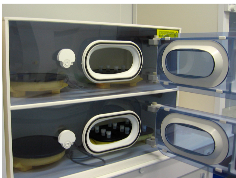
Fig. 24 Hotplates for evaporation in closed system evaporation cabinets with injection of HEPA prefiltered air and independent air exhaustion system (Géosciences Montpellier ultraclean lab).
