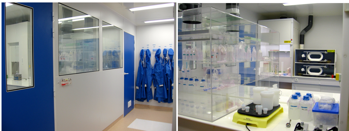
Fig. 22 Overview of the clean lab at Geoscience Montpellier with an 'anteroom' where the precision balance and clean lab-clothes are located (left), and the over-pressurized clean lab (right).
