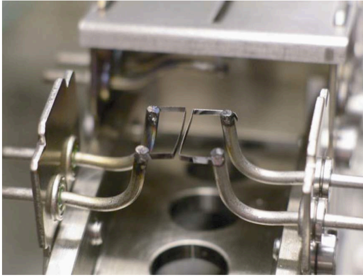
Fig. 28 Re filament ribbons for deposition and loading of samples in TIMS (after Marchesi, 2006; photo by V. Bennett).
