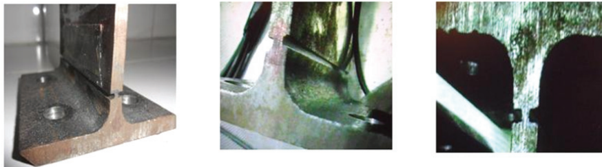
Figura 6.3: Detail of artificial damage made on the I-sections
