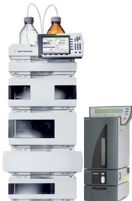
Figure 3.1. Coupling of the capillary HPLC instrument (Agilent technologies) with the LIF detector (Picometrics).
