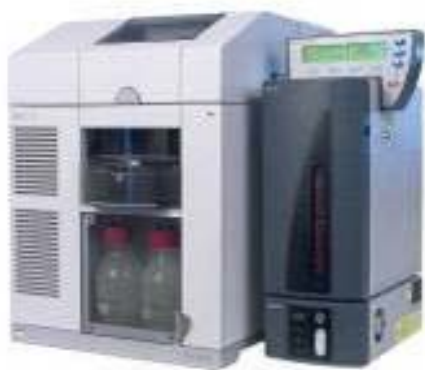
Figure 1.1. Coupling of Agilent CE instruments and Picometrics laser detector.
