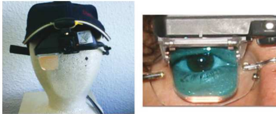
Figure 4: Example of attention application. Figure shows an optoelectronic aid device for low-vision patients. The system includes a camera (scene acquisition) and a wearable processing device that translates the images into useful cues for specific tasks. The attention system may be integrated with this kind of devices to help low-vision patients with tasks such as housework, job controlled environments or even driving scenarios.
