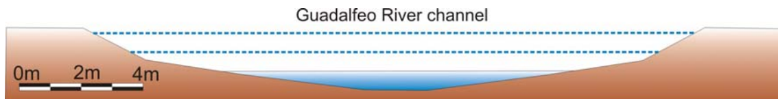
Figure 7. Guadalfeo River channel morphology considered for the SFR package. Discontinuous lines are the potential river stage that can be calculated based on the input parameters.
