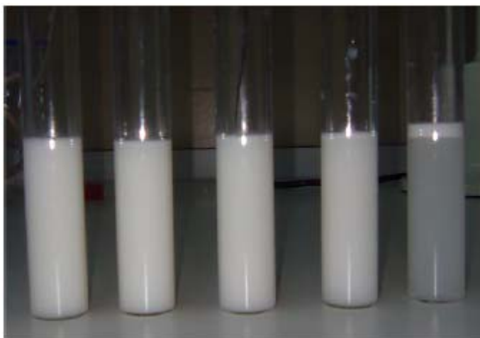
Fig. 1. Oil-in-water emulsion (emulsified with Epikuron) mixed with bile salt NaTDC. NaCl 150 mM. From left to right: [NaTDC]= 0, 0.025, 0.1, 1, 5 % wt. The volume of the sample in the tube is 7 ml.
