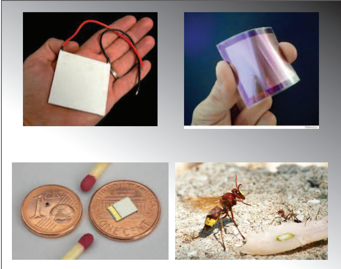
Figure 1.3: Top-left, Peltier cooler composed of thermoelements also shown in picture bottom-left. Top-right, photovoltaic cell. Bottom-right, a photovoltaic-like behavior has recently been observed in the Vespa orientalis hornet. The hornet picture is taken from hornissenschutz.de and the others from several manufacturers.
