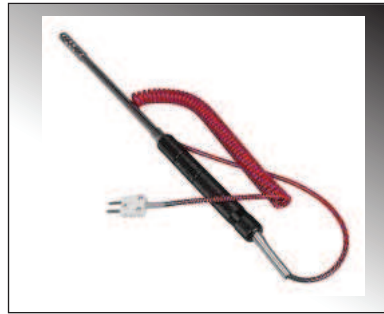
Figure 5.1: Basic thermocouple probe used for the measurement of temperatures, picture taken from www.thermocouples.com/ .
