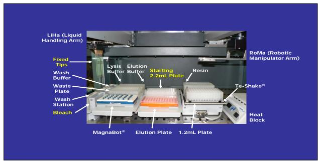
Figure 1. Tecan Freedom EVO® 100 Deck Setup for extraction of DNA from reference buccal samples for both nuclear and mtDNA.
