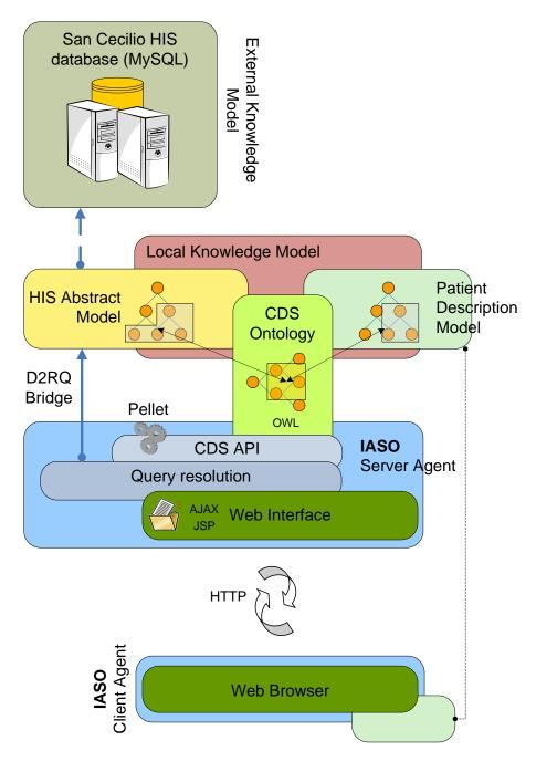
Figure 5.4: Implementation of the IASO prototype
