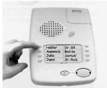
Figure 1. Fixed Telecare Device
