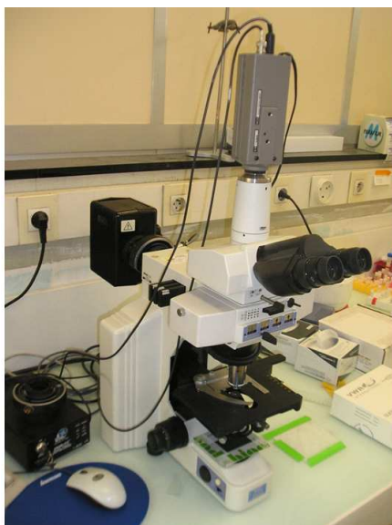
Figure 5.8: Inverted microscope (Leica DM IL) equipped with a Scion CCD video camera and a set of lenses for magnifications of 10, 20, 40 and 100.
