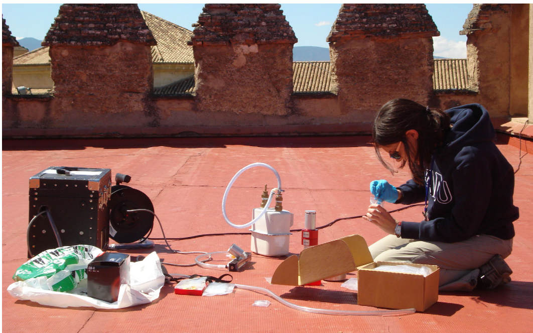
Figure 2. Field work during an aerosol sampling campaign in the Alhambra (Comares Tower).
