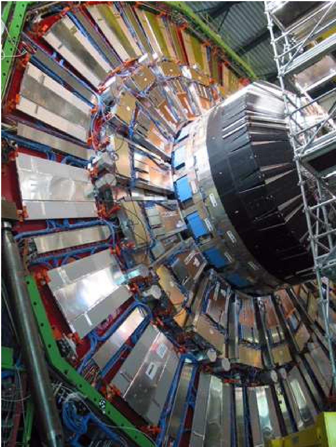
View of one of the end-cap discs installed with muon chambers.
