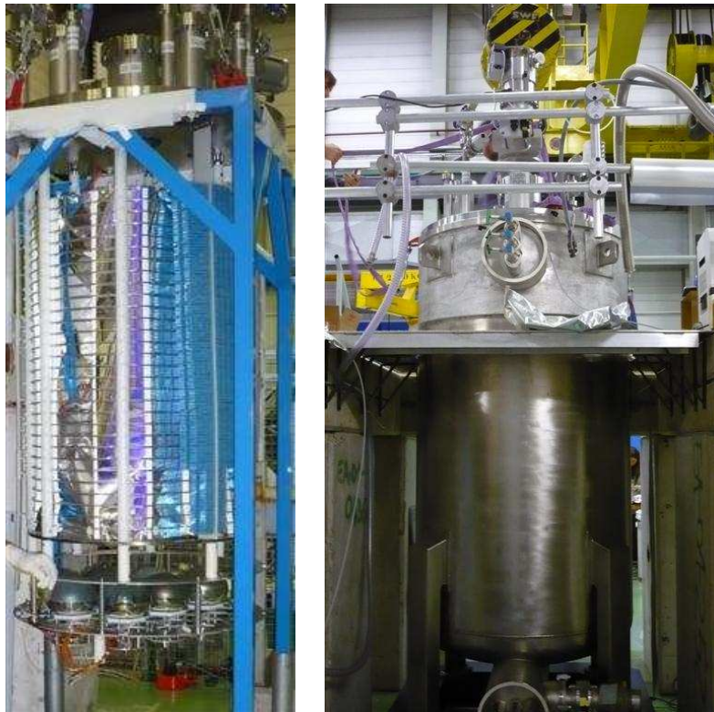
Figure 3.3: Left: Inner ArDM detector. In the image the installed PMTs, field shaping rings and the external part of the wavelength shifter sheets can be seen. Right: ArDM vessel. The empty flange on top connects the vessel with the purification and recirculation systems.
