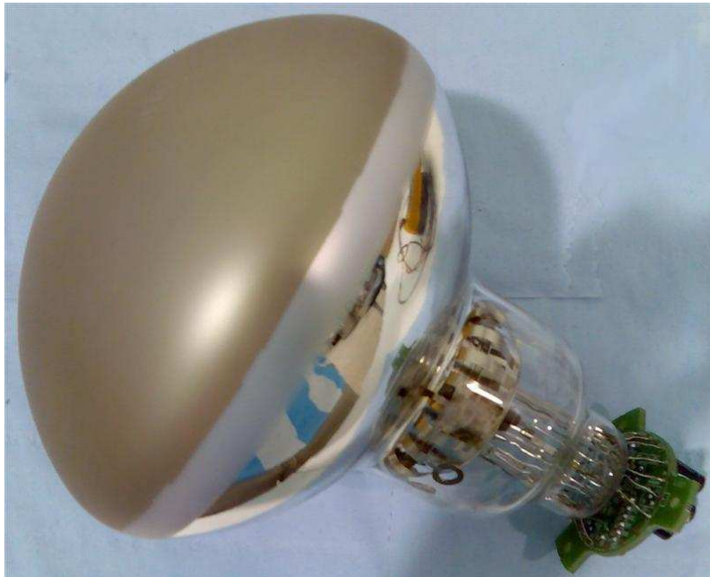
Figure 2.3: Photo of one of 8" PMT tested in this work (ETL9357). The voltage divider can be appreciated soldered to the pins at the bottom of the PMT. The spherical photocathode, on the left, appears covered by the platinum underlayer.
