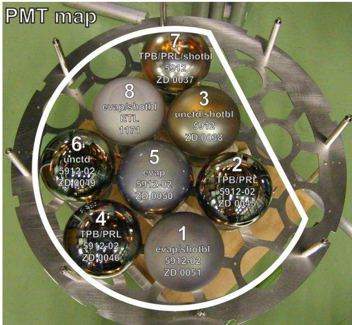
Figure 3.4: Positions of the PMTs during the first surface test in the ArDM experiment. The position of the field shaping rings is marked with a white line. The first line on every PMT refers to the coating procedure (see text) and if the window has been shotblasted. The second line is the PMT model and the third one the serial number.
