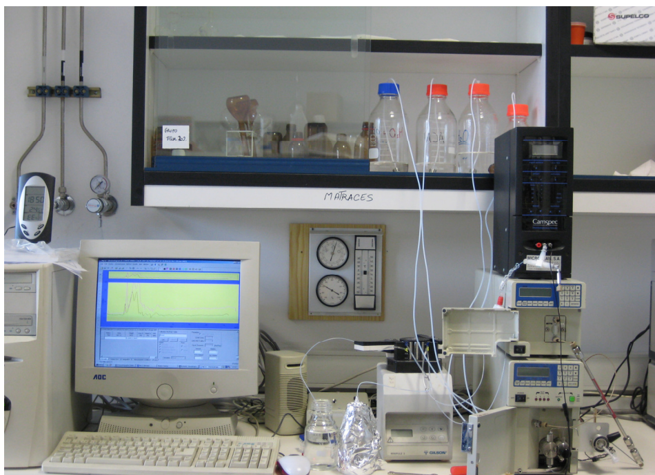
Figure 3.2. HPLC-UV-CL system used in this chapter.
