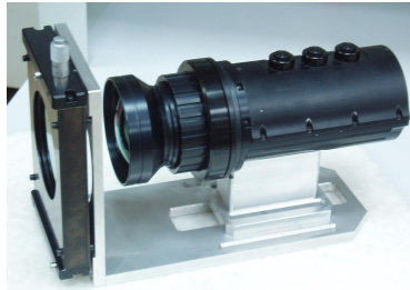
Figure 2. On-axis-coma generator plus conventional thermal camera.
