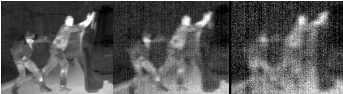
Figure 6: Examples of simulated degradation, including detector noise and optical blur: low degradation (left), realistic simulation (center), and severe degradation (right).
