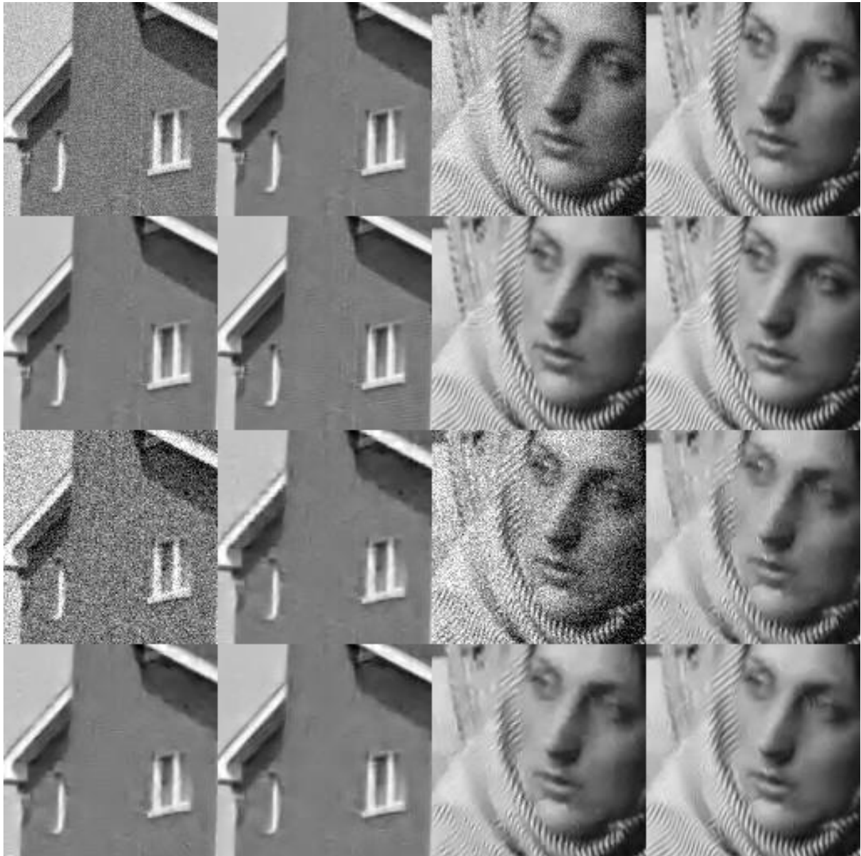
Fig. 4. Visual denoising results using the three compared version of the BLS-GSM denoising method implemented using the translation invariant Haar pyramid (TIHP). For each 2 \times 2 block, up left is the noisy simulated observation; up right is the result with the original BLS-GSM method 3 ; bottom left is the result using the spatially adaptive version 4 ; bottom right is the result using the new multi-GSM model presented here. Upper half correspond to \sigma = 10 and lower half to \sigma = 25 .
