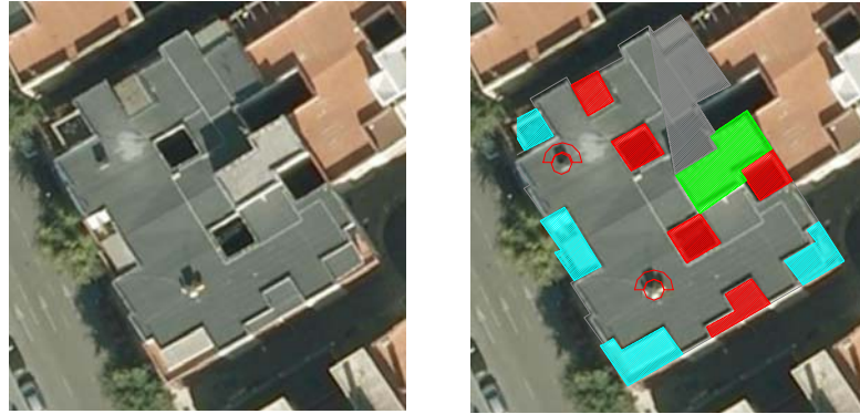
Figures 2 and 3. Calculation of the useful roof surface area, free of obstacles and shading.
