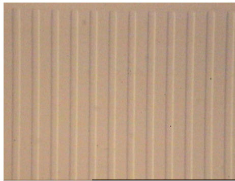
Figure 8.8. Typical optical images of waveguides fabricated by PMMA A9.
