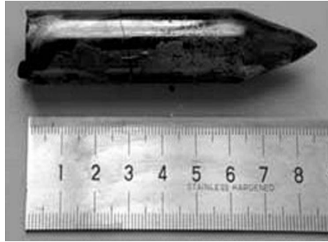
Figure 3.2. CdTe polycrystal ingot growth by Bridgman technique.
