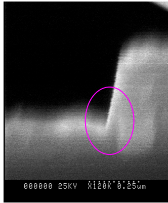
Figure 8.15. Typical trenching effect caused by Ion Milling.
