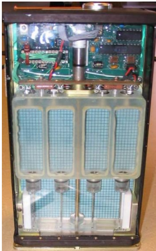
FIGURE 10.1: The experimental apparatus, the Silicate Garden Habitat (SGHab). Developed by BioServe Space Technologies and flown to the International Space Station (ISS) on the space shuttle Endeavour. Dimensions are approximately 10cm width and 20cm height.
