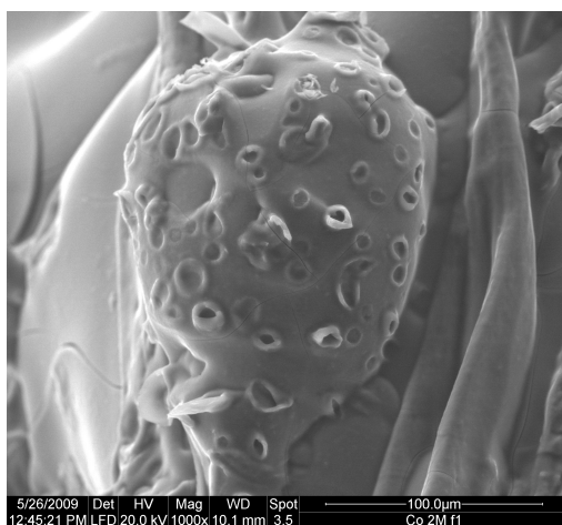
FIGURE 10.4: Micrograph of \text{CoCl}_2 growing in 2 M silicate in microgravity. The beginning of several tubes from the osmotic envelope follow random directions.
