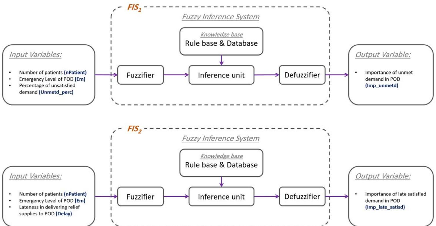
Figure 8: The Proposed FISs' Structure
