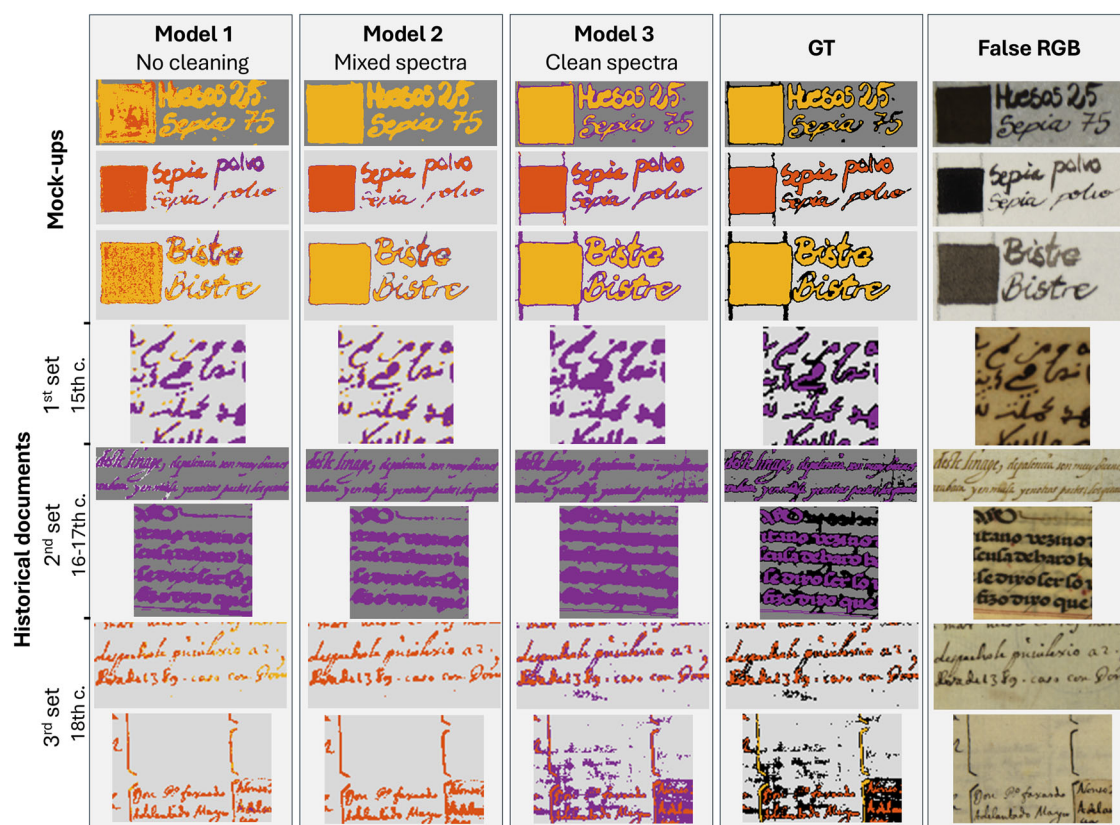
Fig. 3 | Classification maps obtained using SVM models, comparing different spectral processing approaches (Models 1, 2, and 3). Ground Truth (GT) images are shown in column 4, where black pixels indicate uncertain areas. False RGB
