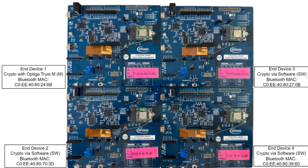
Fig. 17. Testbed used for Secure iBeacon performance measurement.
