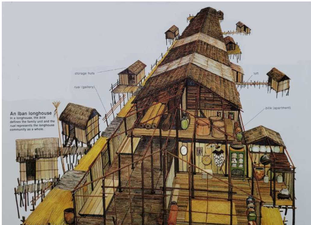
Figure 2. “Sectional Perspective of an Iban longhouse”. Source: Chen Voon Fee, The Encyclopedia of Malaysia: Architecture (New York: Archipelago Press, 1998), 34.
