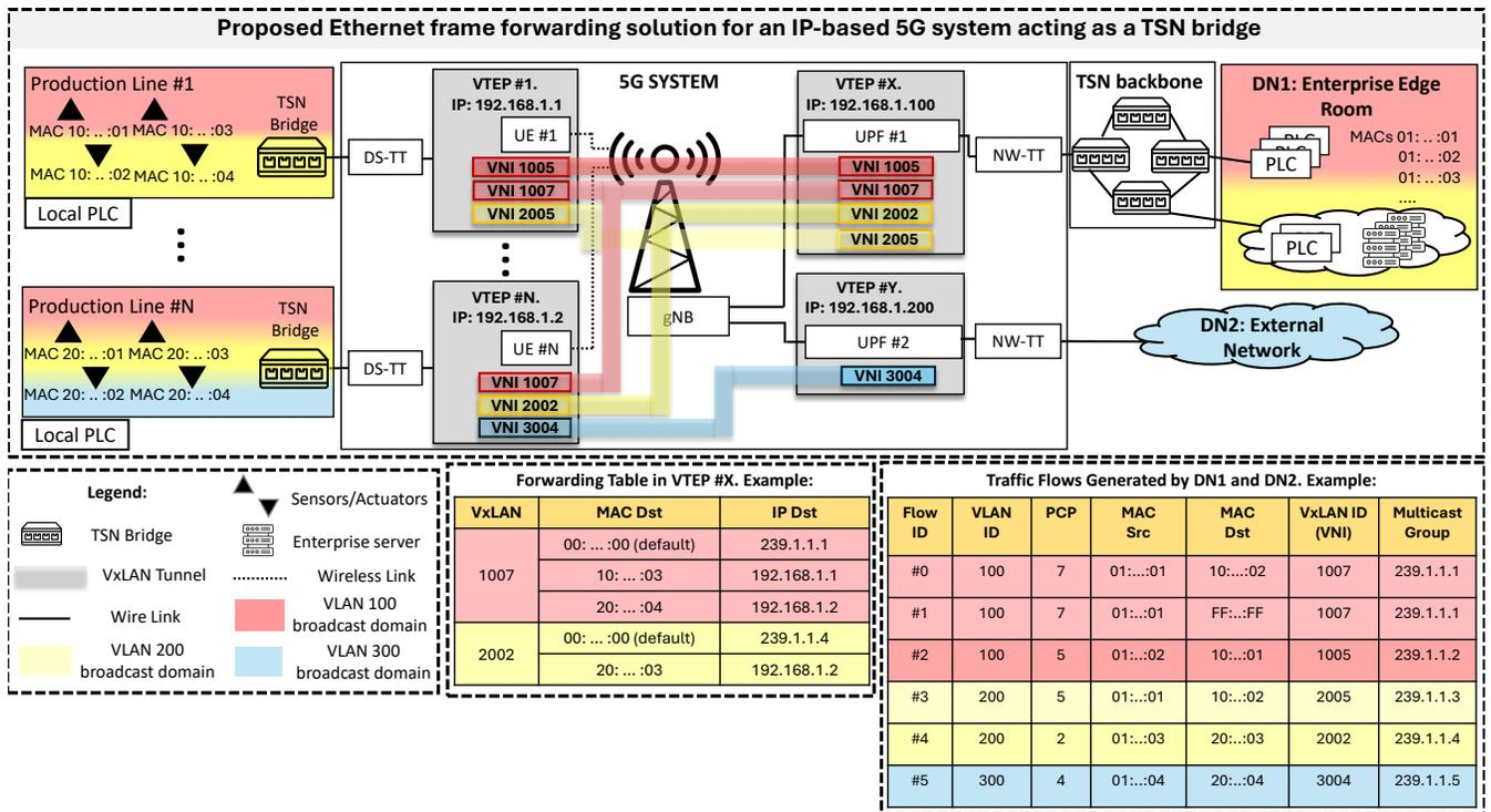
FIGURE 2. Seamless integration of the 5G system into the industrial network via VxLANs.
