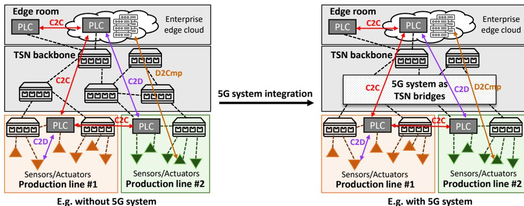
FIGURE 1. TSN-based industrial network in a single-site factory.
