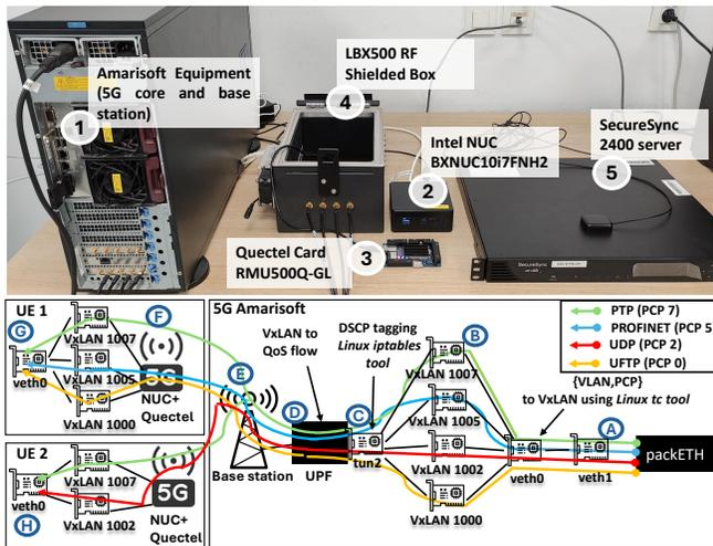
**FIGURE 4.** Proof of concept equipment and evaluated network scenario. To avoid redundancy, only one Intel NUC and one Quectel card, representing a single UE, are depicted in the top image.
