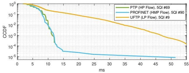
**FIGURE 7. CCDF of the transmission delay of a packet from point A to point G for traffic flows directed to UE 1 (see Fig. 4).**
