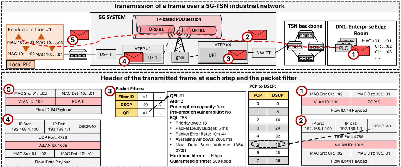
FIGURE 3. Example of mapping a TSN flow into a 5G QoS flow.
