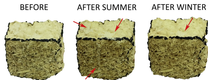
Fig. 6. Appearance of a P sample (CL90S PL + hemp shives mix) before, during and after Mediterranean (Csa) weathering test. Red arrows indicate the presence of white stains. (For interpretation of the references to colour in this figure legend, the reader is referred to the web version of this article.)
