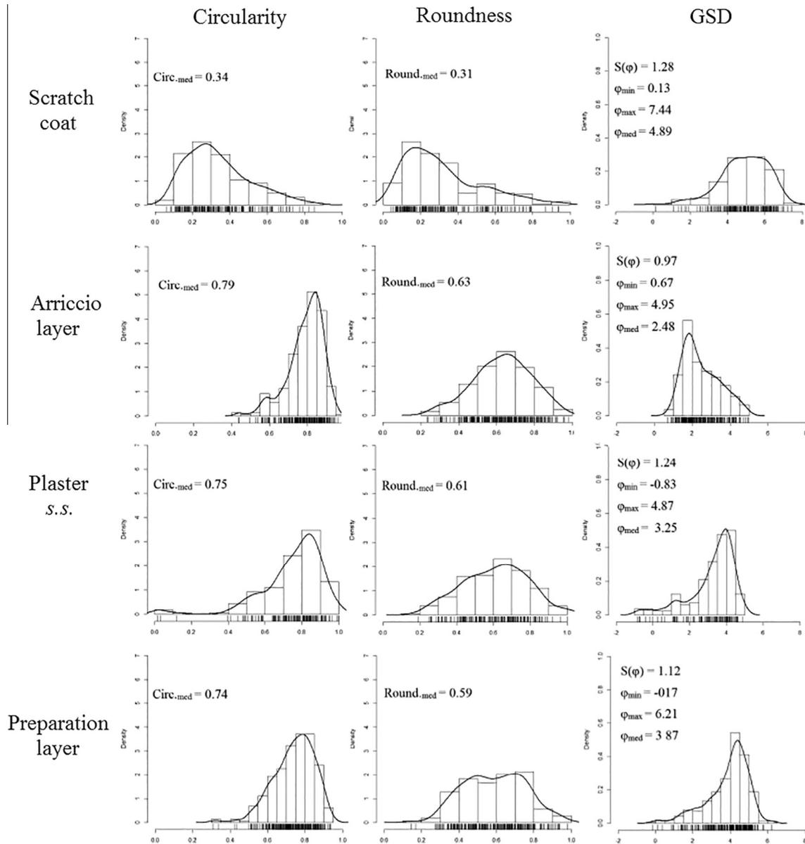
Fig. 6. Density histograms of textural features of the aggregate in sample SM 12: average values of circularity (Circ.) and roundness (Round.), along with statistical descriptors of GSD ( $\varphi$ ) are reported ( $S(\varphi)$  = standard deviation of  $\varphi$  values).
