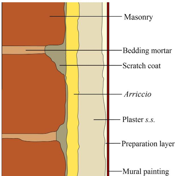
Fig. 4. Sketch section of a typical Roman plaster (inferred from the treatise of Vitruvius [58]).
