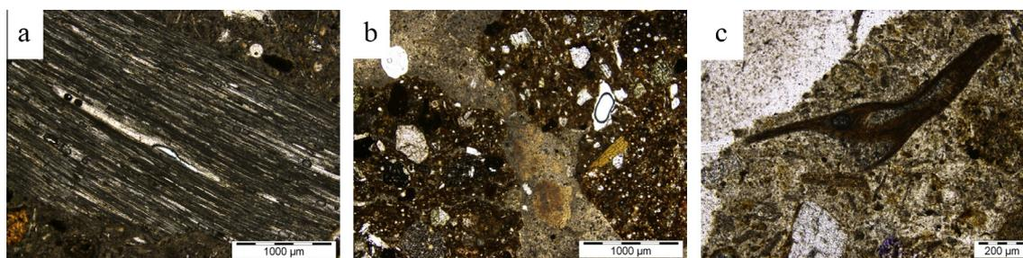
**Fig. 8.** Micrographs of bedding mortars: a) pumice, SM 36, plane polarised light; b) ceramic fragments, SM 38, plane polarised light; c) frustule, SM 40, plane polarised light.
