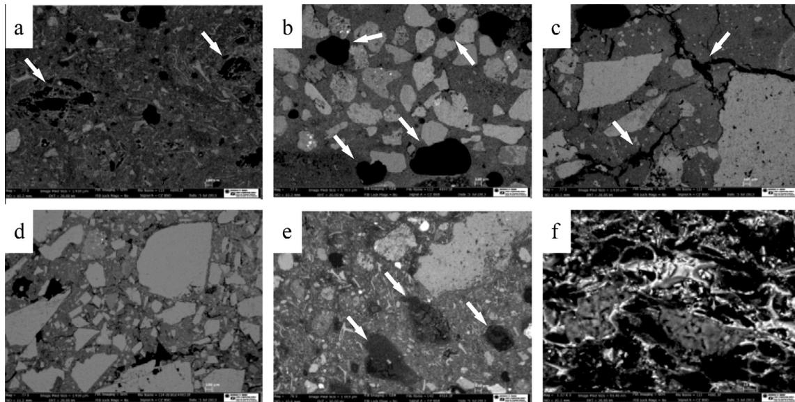
Fig. 13. SEM image and EDS spectra of a reaction lump in the bedding mortar SM 42.
