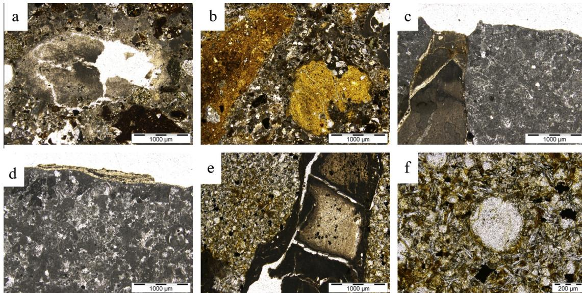
**Fig. 9.** Micrographs mosaics floors: a) unmixed lump with shrinkage fissures in *nucleus*, SM 18, plane polarised light; b) *cocciopesto* in *rudus*, SM 30, plane polarised light; c) *Supranucleus* and limestone white *tesserae*, SM 18, plane polarised light; d) Crust on white *tesserae*, SM 18, plane polarised light; e) *Supranucleus*, SM 30, plane polarised light; f) Leucite-bearing tephritic lava black *tesserae*, SM 30, plane polarised light.
