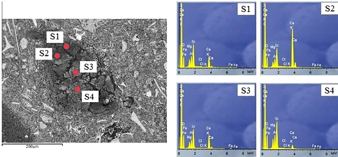
**Fig. 12.** SEM image and EDS spectra along the reaction rim between the ceramic fragments and the binder in a scratch coat SM 12-0.
