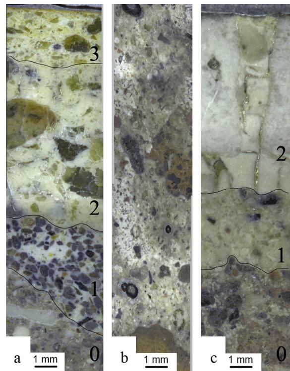
Fig. 5. DVM images of plaster SM 12 (a), bedding mortar SM 38 (b) and mosaic floor SM 30 (c) in which different layers (labelled 0, 1, 2 and 3) can be distinguished.
