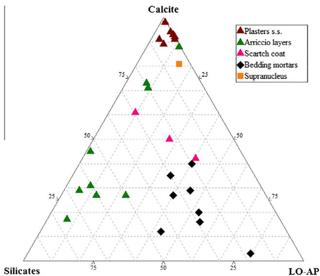
**Fig. 10.** Ternary diagram calcite – silicates – LO-AP (QXPRD).
