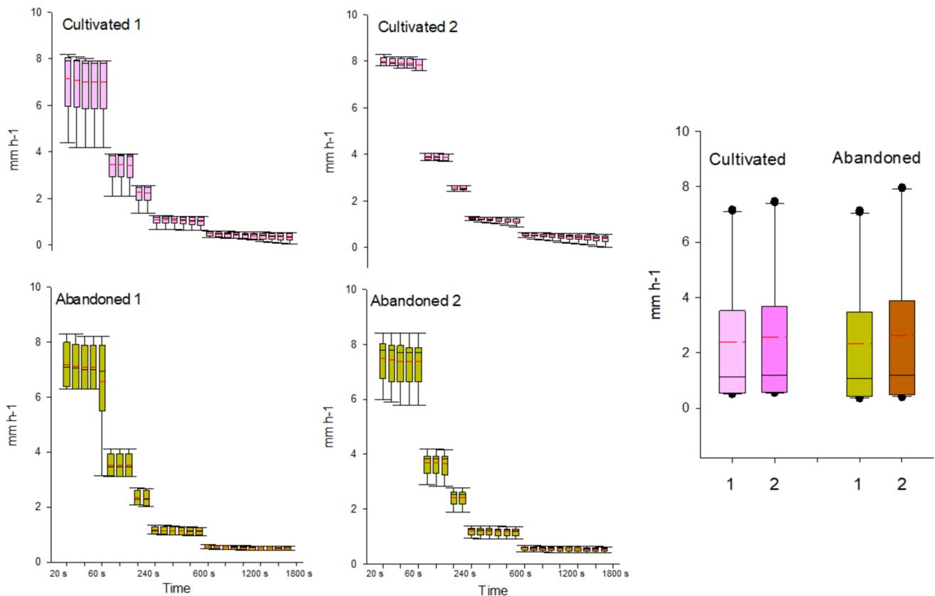
**Fig. 6** Infiltration rates per intervals (seconds) and complete measurements using a mini-disc infiltrometer in both soil managements: cultivated and abandoned with two different repetitions (1 and 2)
