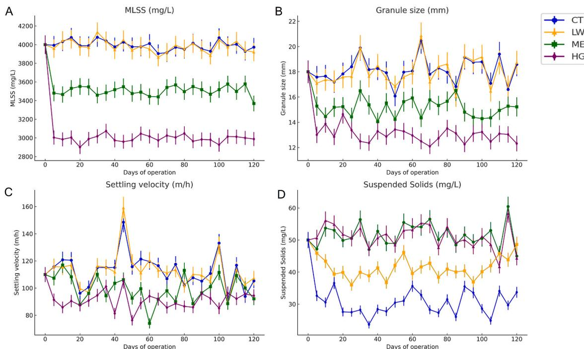
**Fig. 1.** Average MLSS (A), granule size (B), settling velocity of the granules (C) and suspended solids (D) during the experimental period. Treatments consisted of a control without anticancer drugs (CT) and three concentration levels of anticancer drugs classified as low (LW), medium (ME), and high (HG). MLSS, mixed liquor suspended solids.
