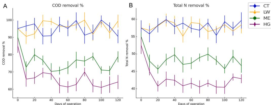
Fig. 2. Average COD removal % (A) and TN removal % (B) during the experimental period. Treatments consisted of a control without anticancer drugs (CT) and three concentration levels of anticancer drugs classified as low (LW), medium (ME), and high (HG). COD, chemical oxygen demand; OM, organic matter, TN, total nitrogen.
