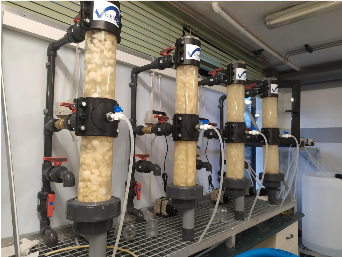
Figure S1: Appearance of granules for each CFR. It can be observed that R1 presented the most defined granules and the clearer water, while the rest of the bioreactors possessed a more disintegrated granules and more turbid water.
