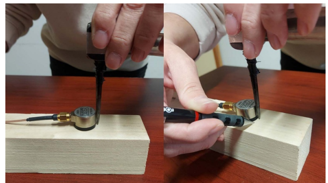
Figure 14. Experimental scenario for measuring the influence of the waveguide of the SD-02 Fakopp sensors.
