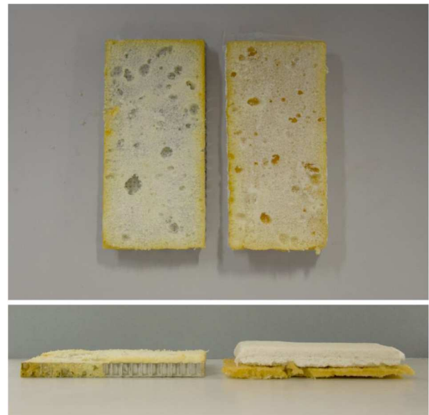
Figure 12. Beva® O.F. Gel + polyurethane foam sample after mechanical separation.
