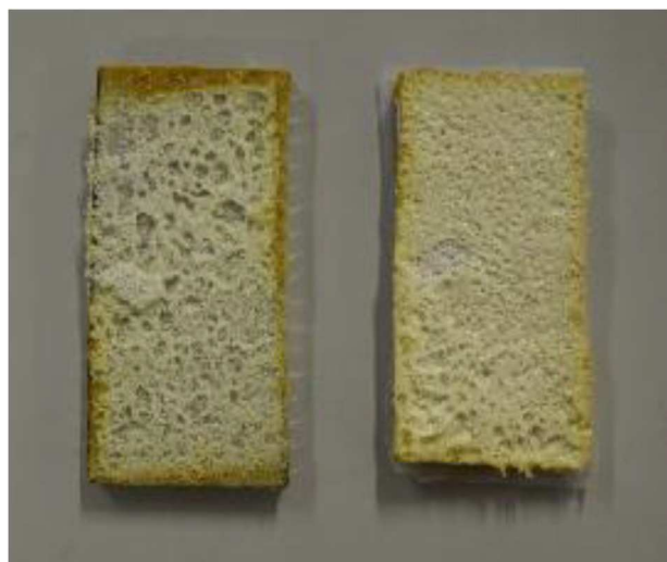
Figure 17. Polyurethane foam specimen used as adhesive and intervention layer after mechanical separation.
