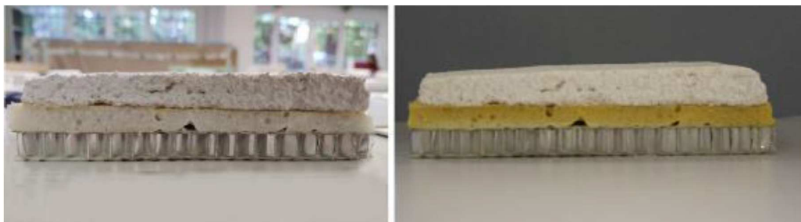
Figure 11. Beva® O.F. Gel + polyurethane foam samples before (left) and after (right) aging.
