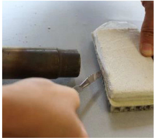
Figure 15. Physical-chemical separation and heat application on epoxy resin and felt sample.
