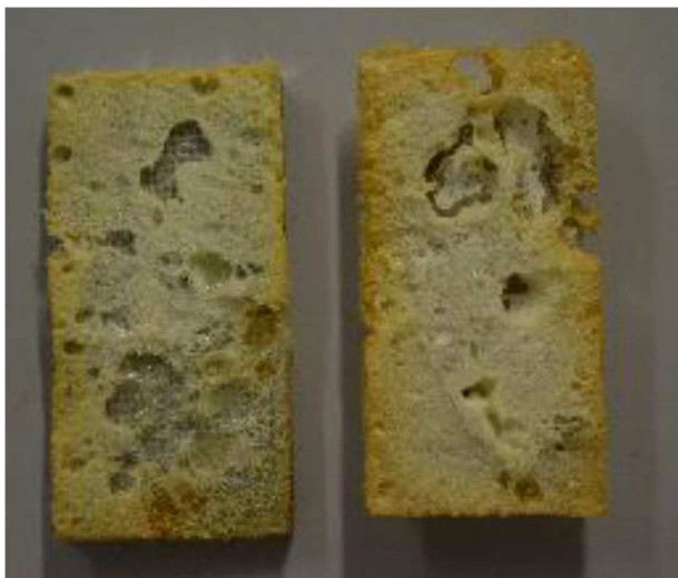
Figure 14. Epo150/K15 + polyurethane foam test specimen after its separation.
