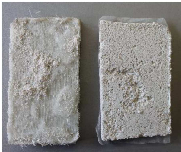
Figure 9. Reverse side of Acril 33 mixed with toluene + gauze test specimen after physical-chemical separation.
