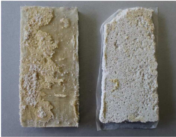
Figure 13. View of the layers in the Beva® O.F. Gel + gauze sample before the separation tests (left) and after separation (right).
