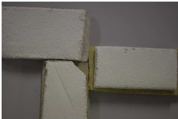
Figure 18. Gauze samples after aging. Top: Acril 33 mixed with toluene. Bottom: Beva® O.F. Gel. Right: Epo 150/K 15.
