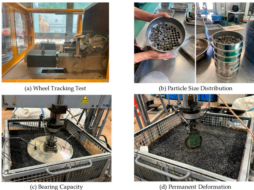
**Figure 4.** Setup of some of the conducted tests.
