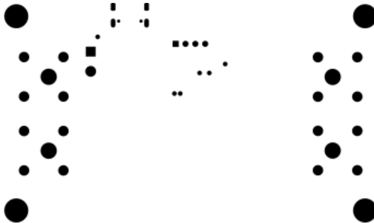
Figura D.3 – Bottom solder mask
