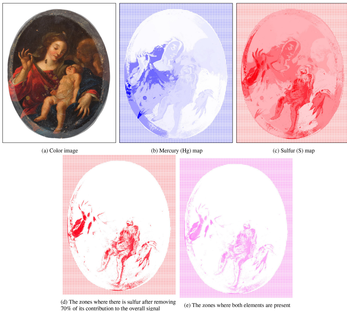
Fig. 5. Operating with maps using “Boceto di Pablo Veronese”: The possible presence of cinnabar can be verified by combining the areas where there is mercury (Hg) and sulfur (S). In this example, we have supposed that 70% of sulfur was combined with calcium (gypsum), leaving 30% to combine with mercury. The area with a grid indicates that there are no valid values.
