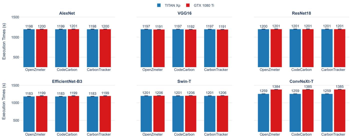
**Figure 8.** Average Execution times (s) during the training of AlexNet, VGG16, ResNet18, EfficientNet-B3, Swin-T, and ConvNeXt-T on GPUs TITAN Xp and GTX 1080 Ti. The graph compares the results from three energy measurement tools: OpenZmeter (energy meter reference), CodeCarbon, and Carbontracker.
