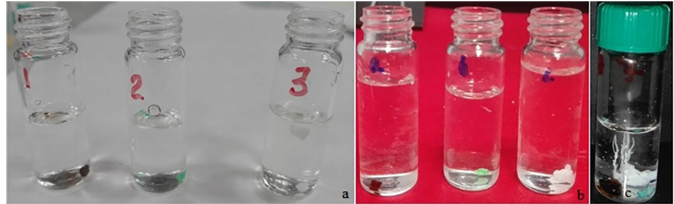
Fig 1. Perchlorate gardens in the solid-liquid phase: (a) Experiment B, \text{FeSO}_4 \cdot 7\text{H}_2\text{O} , \text{NiSO}_4 \cdot 7\text{H}_2\text{O} and \text{CaCl}_2 salts at 3M of sodium perchlorate (1, 2 and 3 labels respectively) (b) Pellet method and 2M concentration (Experiment C), with the same order as experiment B and (c) Experiment E. White, brown and green correspond to the structures of \text{Ca}^{2+} , \text{Fe}^{2+} and \text{Ni}^{2+} salts respectively.
