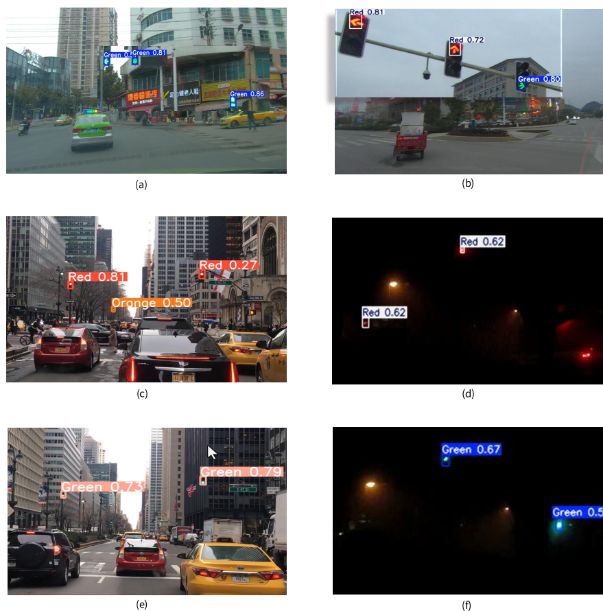
Figure 13. The performance of Meta-YOLOv8 is demonstrated under various conditions, including different ranges and lighting scenarios: (a) effectiveness in bright daylight from approximately 200 m away, and (b) functionality in low light compared to a clear day (cloudy evening) from around 150 m from the driver's perspective. In both cases, traffic lights are accurately detected from a long range. Additionally, images (c,e) show testing in a morning light environment from approximately 200 m and 170 m, respectively. Images (d,f) depict a complete night-time scene, demonstrating the model's ability to detect and differentiate between street lights and traffic signals under challenging conditions with faint and glaring lights from an approximate distance of 50–65 m.
