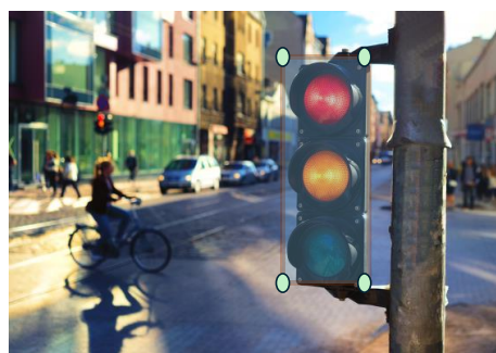
Figure 6. Conventional labeling, where bounding box covers entire traffic light, in which 1/3 of object area does not impact the learning process.
