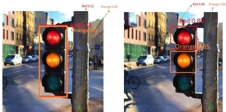
Figure 12. Meta-YOLOv8 (b) with new labeling exhibits superior detection capabilities relative to YOLOv8 (a) with conventional labeling, effectively minimizing ambiguity and precisely differentiating among various colors within a single frame devoid of overlap. YOLOv8 (a) uses overlapping bounding boxes, while Meta-YOLOv8 (b) displays a distinct delineation of colors, ensuring clarity for both observers and automated systems, thereby eliminating potential confusion.
