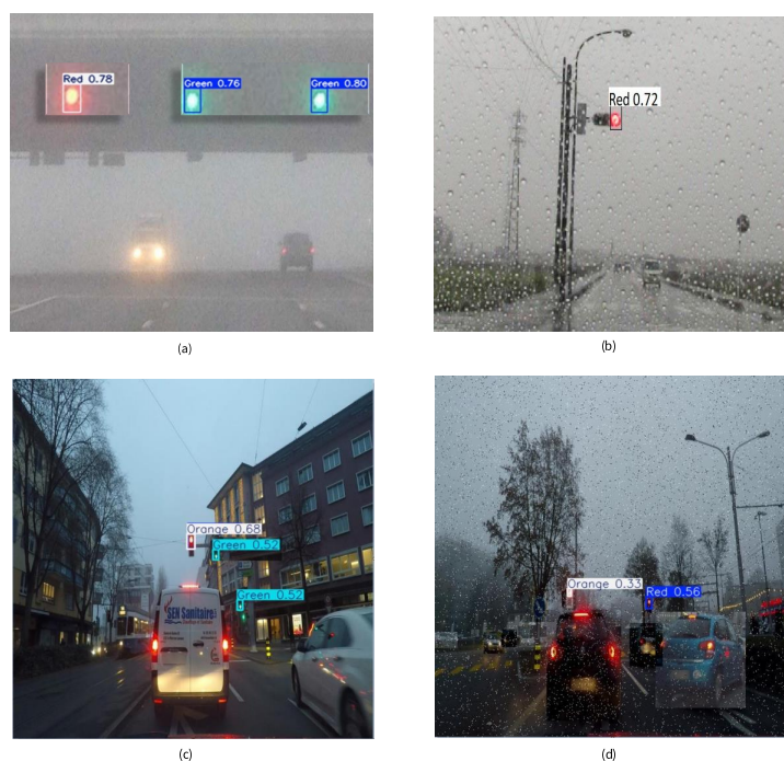
Figure 14. Adaptability performance evaluation of Meta-YOLOv8 in adverse weather: (a,c) Detection capability during dense fog at approximately 55 and 75 m, respectively, and (b,d) operational efficiency in intense rain at approximately 60 and 70 m, respectively, from the driver’s viewpoint.
